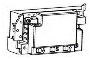
The switch in the upper left corner of the LCD is to select input control signal type: C for  $0/4\sim20$ mA and V for  $0/2\sim10$ V. Furthermore, selection should be done with buttons to set the minimum control signal (0 or higher).
