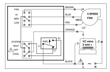
Fig. 6b - T6069A, 5-wire for single "VC" series ( 2 wire + common ) valve, cycled fan, manual heat / cool changeover.
