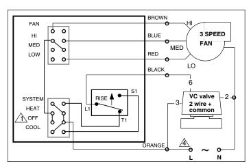
Fig. 6a - T6069A, 5-wire for single "VC" series ( 2 wire + common version ) valve, constant fan, manual heat / cool changeover.
