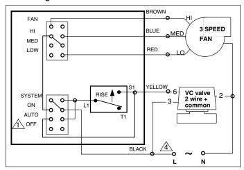
Fig. 10 - T6069E, 5-wire for single "VC" series valve( 2 wire + common version), constant or cycled fan, cooling only.
