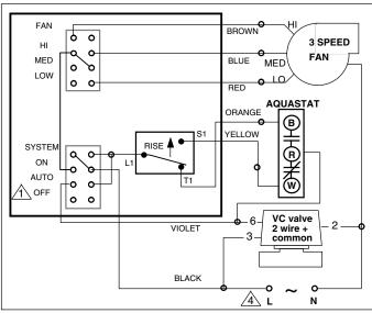
Fig. 9 - T6069D, 7-wire for single "VC" series valve (2 wire+common version), constant or cycled fan, auto heat / cool changeover.
