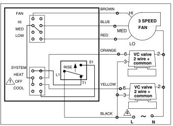
Fig. 8a - T6069C, 6-wire for dual "VC" serie valve ( 2 wire + common version ), cycled fan, manual heat / cool changeover.
