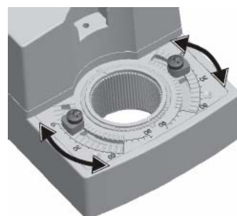
Fig. 5. Mechanical end limits
