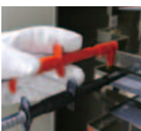
For clamping around the target busbar
