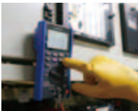
Press the MEM key to save measured values in the instrument's internal memory.
