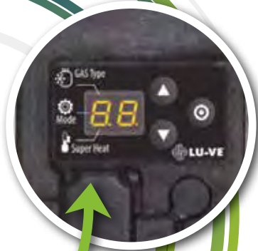
Display for setting working parameters.
