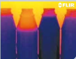
Thermal image shows bottles that are over- or under-filled.
