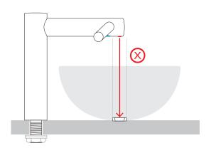
**Fig.3** Minimum distance from tap centre to top of sink (AB11 only) 100mm. Front edge of sink (all types – pedestal, recessed, slab) to wall minimum 385mm.
